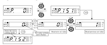
Note: At the parameter setting mode, both the indicating lamp of Hz and MON will be off. Please make sure to hold down the key for more than 0.5s when writing for the set value of the parameters.
