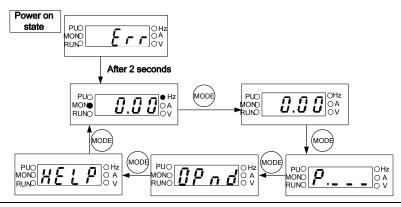
Note: 1. For detailed operating flow at monitoring mode, please refer to Section 4.1.3 of SS2 series inverter instruction manual.
